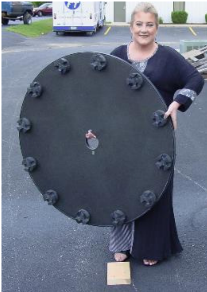
A 42" Diameter Carbon Dial Indexing Table with 12 stations. The tooling station nests are also composite.
