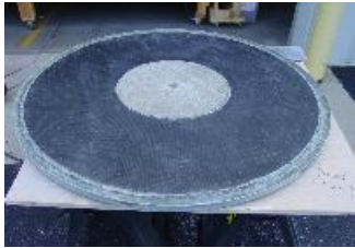
Special Carbon Dial Table with Reinforced Glass-Fiber edge for tool mounting.
