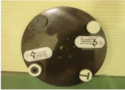
30in Carbon Dial table with composite tooling.
