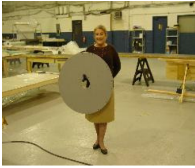
A 15lb Ribbed Carbon Fiber Dial Table, Coated with Polane. The dial table is a replacement for an existing aluminum dial table at a automotive clients facility.
