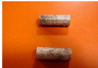
STEP 1: Aluminum knurled inserts as provided from manufacturer. Insert body contaminated from oil and handling.
