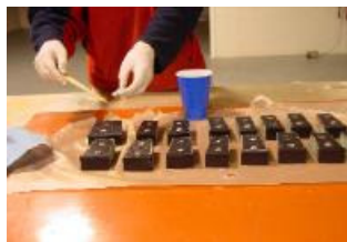
STEP 5: Epoxy Adhesive applied to surface of insert
