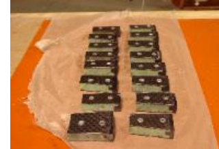
STEP 6: Inserts potted in Carbon Dial table samples. Wait 24 hours before machining
